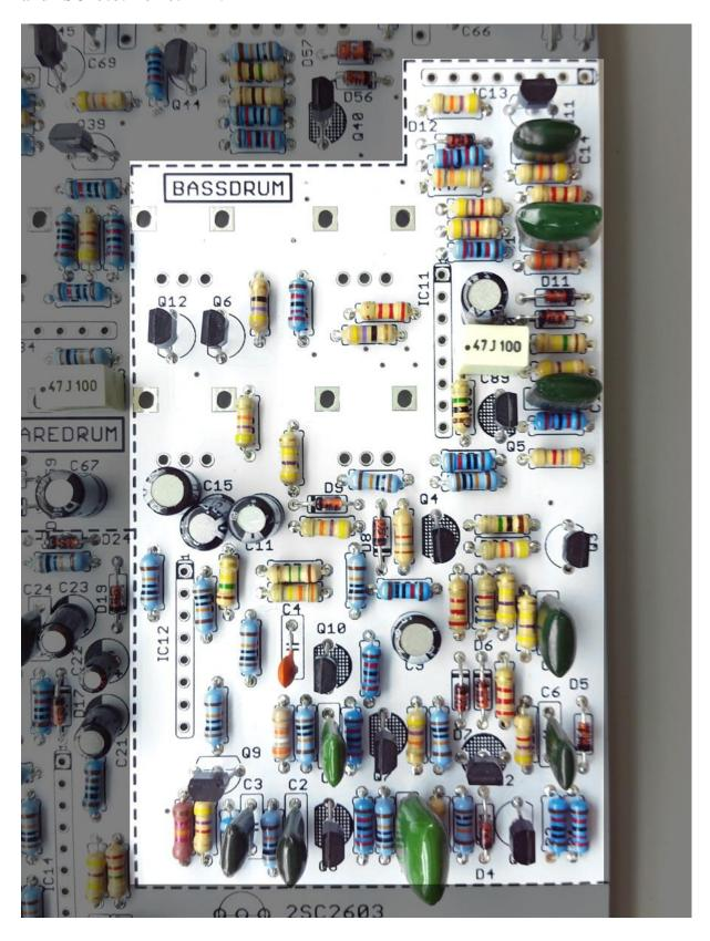
Now, check bassdrum section power voltages and add ICs. **Do not overheat ICs pins during solder process!**
