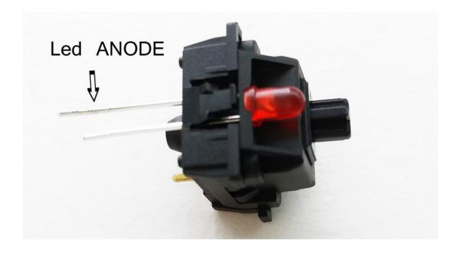
Add switches. Pay attention to orientation of which you solder switches. Long legs must match with positive symbol on the silkscreen.
