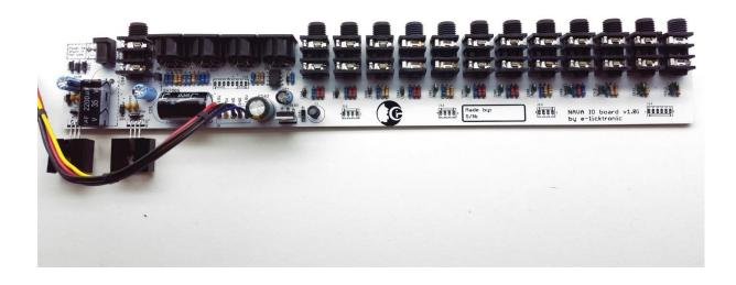
Now, check io board section power voltages and add the 6N138. **Do not overheat ICs pins during solder process!**
